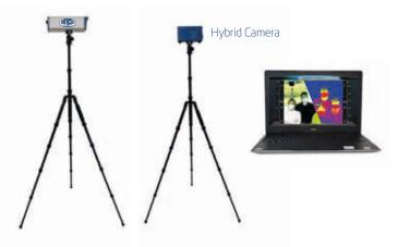
The new technology we are proposing allows a very precise temperature measurement (accuracy up to +/-0.3 °C or +/-0.2°C). In addition, these cameras produces a simultaneous analysis of up to 30 faces and the results are shown in few seconds.
