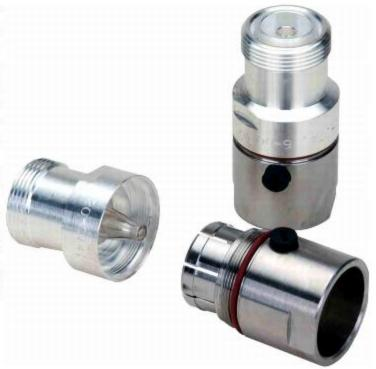
Moreover for the largerly used 1/4", 3/8", and 1/2" coaxial cables "monolithic" connectors have been designed in order to avoid intermodulation products normally caused by mechanically most complex connectors.
